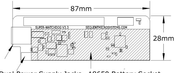
Dual Power Supply Jacks 18650 Battery Socket
